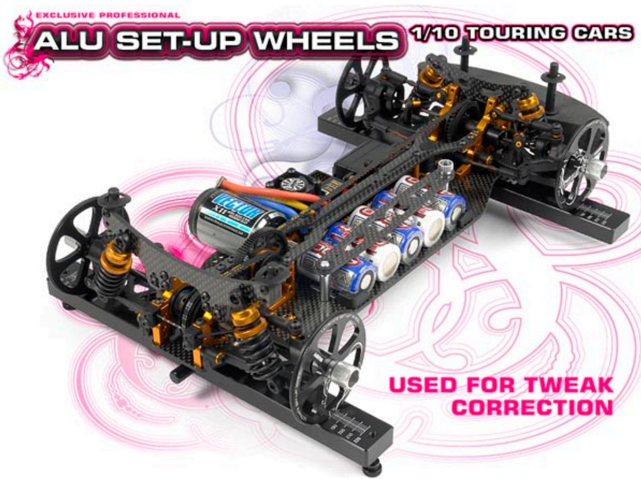
When checking tweak on a foam-tired touring car, the differences between tires are even greater than with rubber tires. Each foam tire has a different diameter after each run due to tire wear, making it impossible to check for tweak because the tires can give very misleading results. In this case the alu set-up wheels are the best tool for checking tweak.
