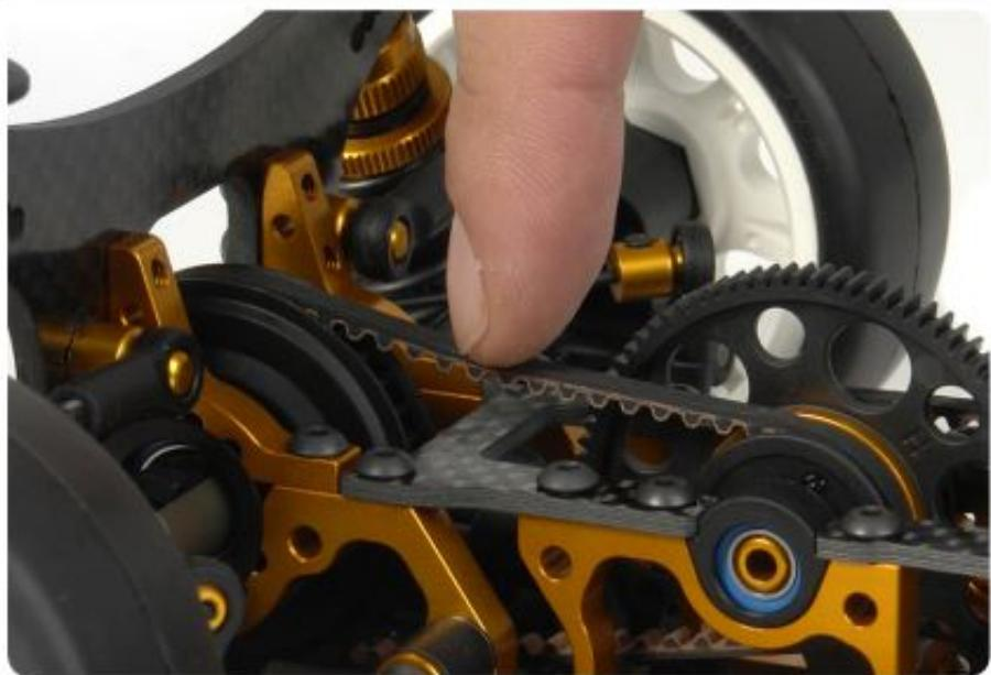
When the belts are mounted in the car for the first time, they will be tighter than the standard belts. Therefore we recommend you adjust the eccentric bushings so that the belts are slightly looser, though it may happen that the belts still feel a bit tighter. Note that you can also use the #302077 1mm composite hubs for bulkheads to reduce the belt tension. The tension of the belts will not have a negative effect on the car's performance, and the belts will become softer after some run time.
